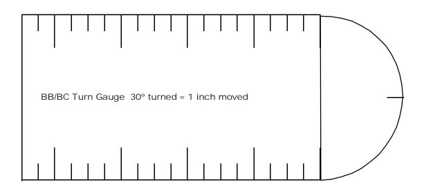
Note: Mark the semicircular ends of the turn gauges in 30 degree increments.
